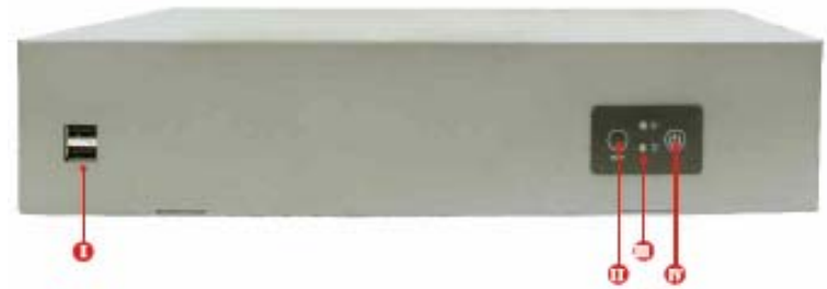
I. USB Port II. Power Reset Button III. Power / HDD LED IV. Power On Button
